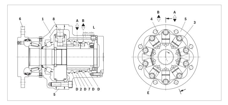
Hydraulic motors of the type MCR-F are radial piston motors with rear case mounting and flange shaft. The MCR-F motors are intended for wheel drives in open or closed circuits. These motors are used in a wide range of applications such as municipal vehicles, fork lift trucks, agricultural and forestry machines. The integrated flange with wheel studs allows easy installation of standard wheel rims.
