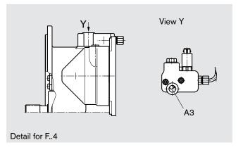
For technical data, see table of values on page 6. The pressure-relief valve installed to protect the integrated auxiliary pump has a fixed setting of 30 bar. An electrically controlled pressure-reduction valve can be used to override the power setting (load-limiting control).
