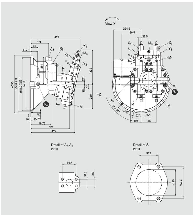
R -Must be connected to tank to ensure cooling and lubrication of bearing sets.
