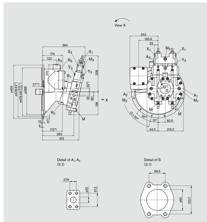
\*) Center of gravity \*\*) with auxiliary pump 10.7 cm<sup>3</sup> = 4.7 mm
