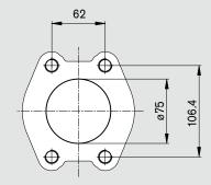
1) Dimensions according to SAE J617-No. 4, for connection to flywheel case in internal combustion engine.
