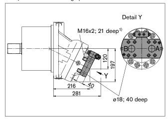
Port plate 107 - SAE flange ports at bottom
