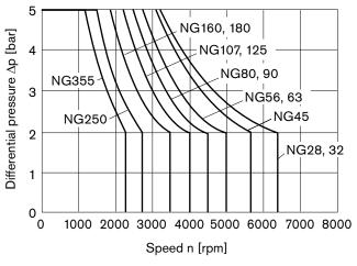
The values are valid for an ambient pressure  $p_{abs} = 1$  bar.
