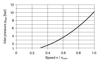
This diagram is valid only for the optimum viscosity range from  $v_{\text{opt}}$  = 36 to 16 mm²/s.
